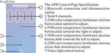
2. Total 8 channels. 3.3200 color temperature luminance increased button, slide upward to adjust.
