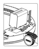
3. When removing the lithium batteries, please press the battery lock and then take out the lithium batteries
